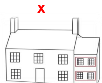
Side extension: windows of wrong proportion
