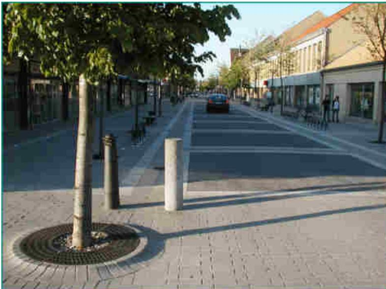
**Figure 7.2:** An example of a “shared surface” within a town centre, with subtle changes in the colour/sizing/alignment of paving to denote vehicular/pedestrian routes, and the use of soft landscaping etc... as “natural” traffic calming (Source: <http://www.hamilton-baillie.co.uk/gallery.htm>)
