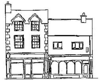
**Fig 6.2:** Where a single shop occupies two buildings, appropriate variations in shop front design coupled with changes in fascia levels can emphasise the buildings’ individuality, thus retaining the traditional “rhythm” of the streetscape.
