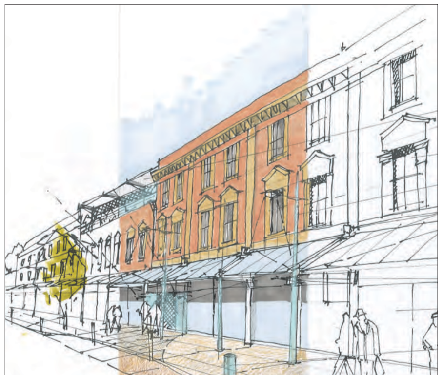
Figure 40: East (lower) Bethcar Street re-elevated with glazed canopies to shop fronts
